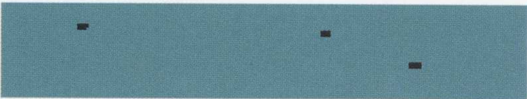
0.3% Coating Breakdown
